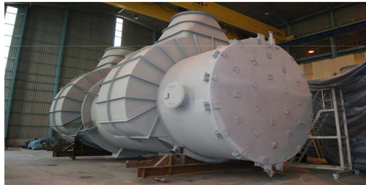
Client SNC Lavalin / JPMC, 2.011. Material SA-516 Gr. 70 + 304 Weight 135 mT Length 14.500 mm Diameter 4.800 mm Thickness 8600mm
