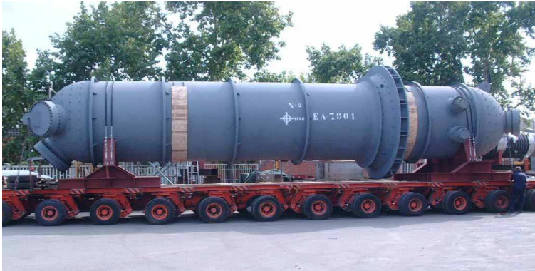
Client Alfa Laval Packinox, 2.005 Material SA-387 Gr.11 Cl2. Weight 115mT Length 12.500 mm Diameter 2.400 mm Thickness 70 mm
