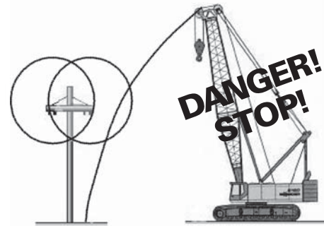
This crane boom could reach within the minimum distance.
